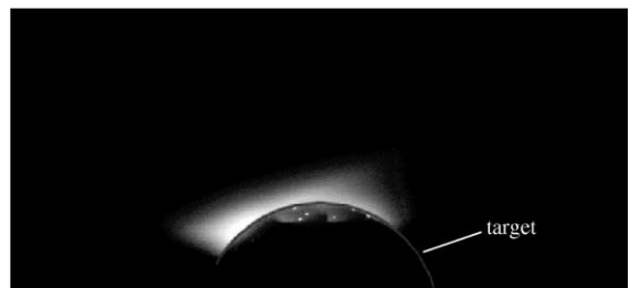
Fig. 5. Side view of the carbon target with H\alpha filter during discharge
